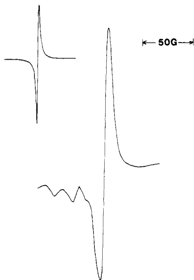
Figure 9. ESR spectrum of oxidized (TPP)InMo(CO) 3 Cp at 120 K in CH 2 Cl 2 containing 0.1 M (TBA)PF 6 .
